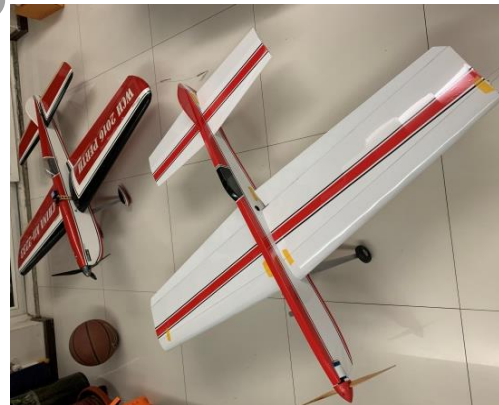
Fig. 4.9 - The model plane with the removable leading edge
