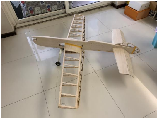
Fig. 4.7 - The model plane before final cover
