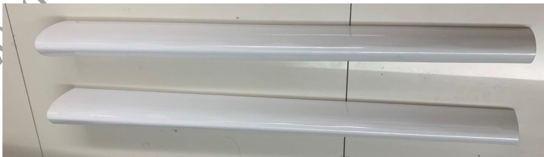
Fig. 4.10 - The removable straight leading edge
