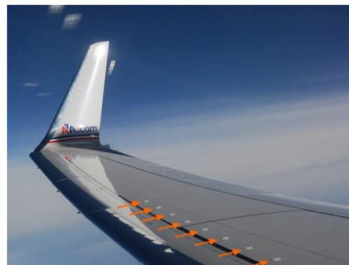
Fig 1.5 - Vortex Generator on Bone 737 [1]
