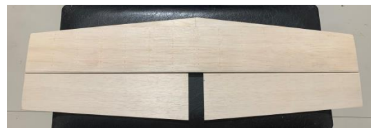
Fig. 4.6 - Stabilizer and elevator
