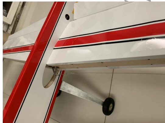
Fig. 4.8 - The model plane after cover (without leading edge)
