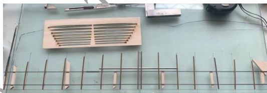
Fig. 4.6 - Stabilizer and elevator
