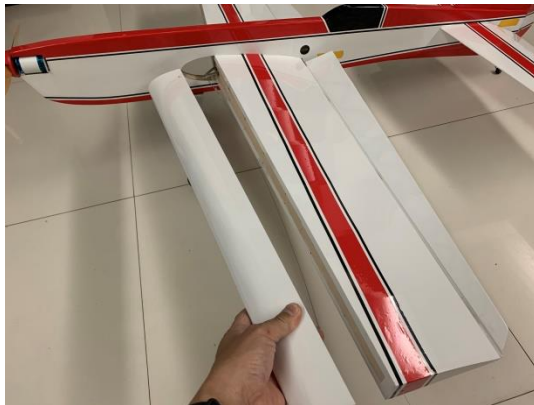
Fig. 4.9 - The model plane with the removable leading edge
