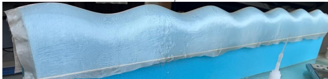
Fig. 4.17 – cover with fiberglass
