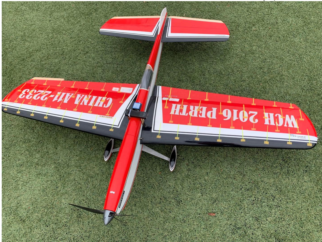
Fig. 1.2 - Control line air model plane that I flew in the 2016 World Championship (To note, the thin yellow stripes and tapes are not part the original model. Those are temporarily fixed onto the wing in order to observe the air flow during flight, and to visualize possible stalls during maneuver.)
