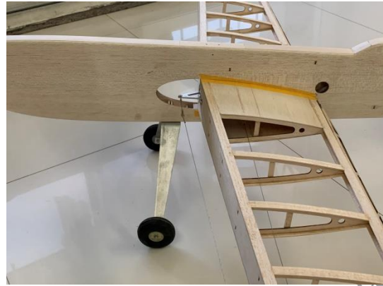
Fig. 4.7 - The model plane before final cover
