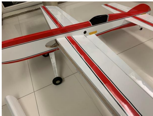
Fig. 4.8 - The model plane after cover (without leading edge)
