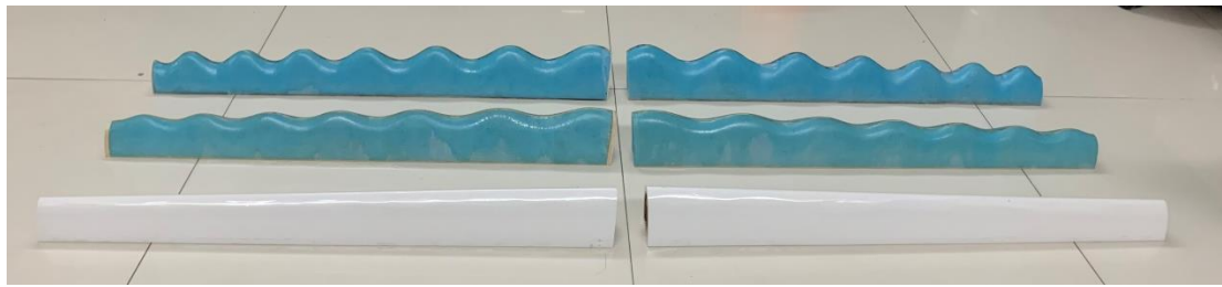
Fig. 4.20 – 3 different type of leading-edge have been tested
