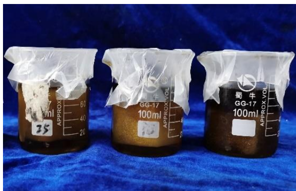
Figure 2: PU sponges immersed in the mixture of DA, PEPA and Tris solution.
