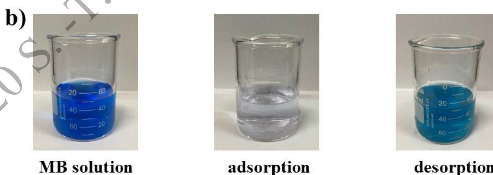
Figure 12: The adsorption and desorption for the decorated sponge of MB in acidic/alkaline conditions: (a) surface chemical structures; (b) color changes.
