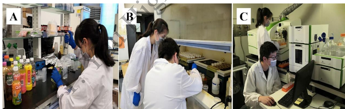
Figure 2.1 Extraction process of Sb: (A) pipetting samples; (B) digestion on a hotplate; (C) determination of Sb by ICP-MS.
