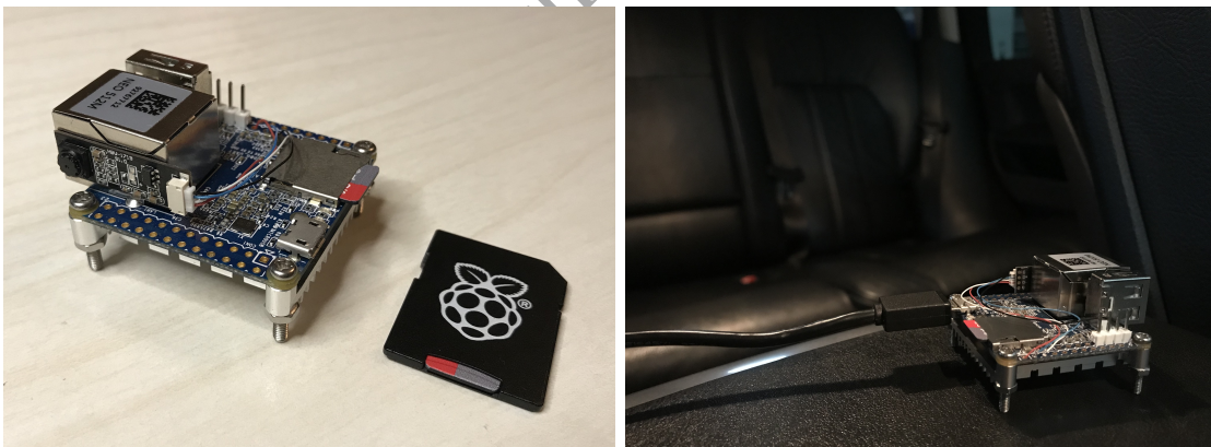
Figure 7: Left: Embedded device prototype (SD card for size reference). The SMS module (not visible) is located under the board. Right: The device is positioned on the center console of the car, facing the backseat. It is powered through the car's auxiliary power outlet.
