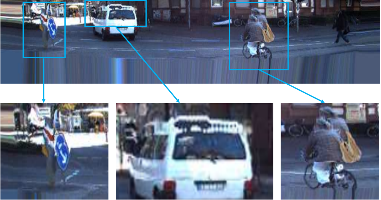
Figure 3. The artifacts produced by FuseSeg[7]. There are noticeable ghosting such as around the cyclist.
