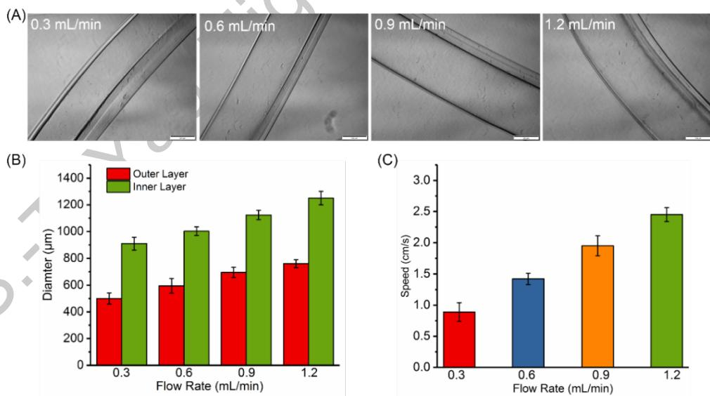
**Figure 3.** Characterization of alginate hollow tubes: (A) bright-field images of the tube fabricated at different flow rates (scale bar is  $500 \mu\text{m}$ ), (B) relation between flow rate and tube diameter, and (C) Relation between flow rate and printing speed.
