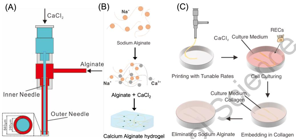
**Figure 2.** Schematic of the construction of the FSSRT: (A) schematic of the coaxial device, (B) formation of calcium alginate hydrogel, and (C) main experimental procedure.
