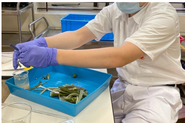
Picture 2: extracting the okra mucilage from its central axis
