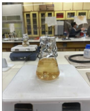
Picture 18: Cu with starch (capping agent) and L-ascorbic acid (reducing agent); Left: right after the complete addition of all reactants; Right: the solution after 1 hour of stirring and heating.
