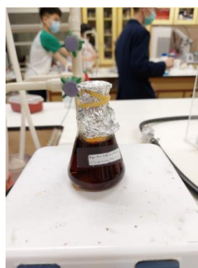
Picture 41: Cu with cysteine (capping agent) and glucose (reducing agent), before and after addition of the copper ion solution.
