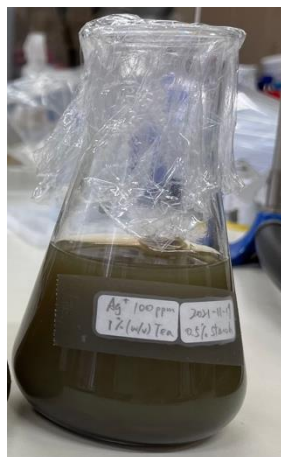
Picture 7: starch-capped and tea-extract-reduced Ag mixture
