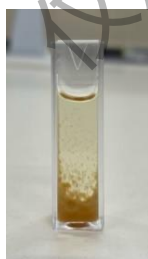
Picture 27: Chitosan/AgNPs precipitated out in LB.
