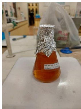
Picture 19: Cu with chitosan (capping agent) and L-ascorbic acid (reducing agent).
