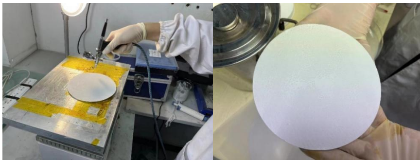
Figure 15. The dry-cleaned glass fiber is sprayed and coated, during which the clear spraying equipment is changed 3 times
