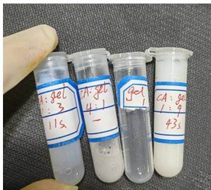
Figure 7. When the ratio of solution B to solution A exceeds 4:1, a relatively thin solution is formed
