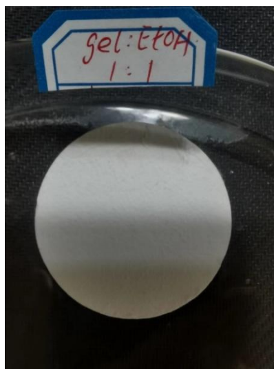
Figure 9. The dripping effect of the original system solution with equal proportion of anhydrous ethanol, which is obviously different from the dripping effect of pure solution.
