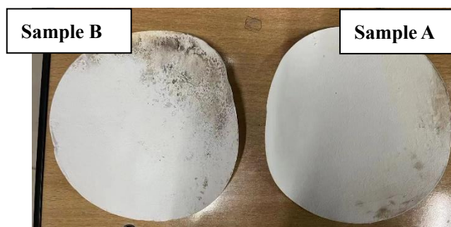
Figure 16. Product A obtained by spray coating (on the right) exhibits fewer yellow-black spots in its distribution, while product B obtained by coating (on the left) shows more black spots.
