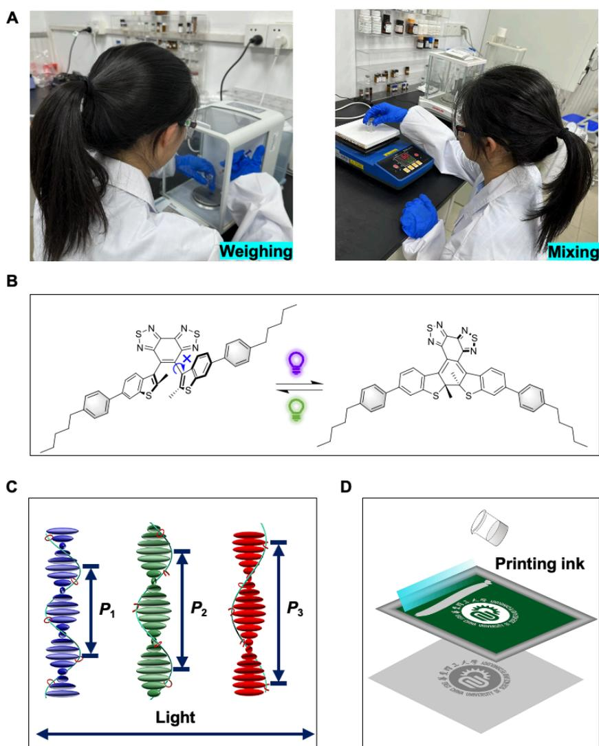
**Figure 2.1 Photoprogramming of printing ink with suitable viscosity and broad-range structure color.** (A) The researcher is weighing and mixing the substances. (B) The structural change of DAE under UV light and visible light. (C) The change of the helical pitch in the LC system under UV light irradiation. (D) Printing ink is added to the LC system so that patterns can be painted on a flexible substrate.
