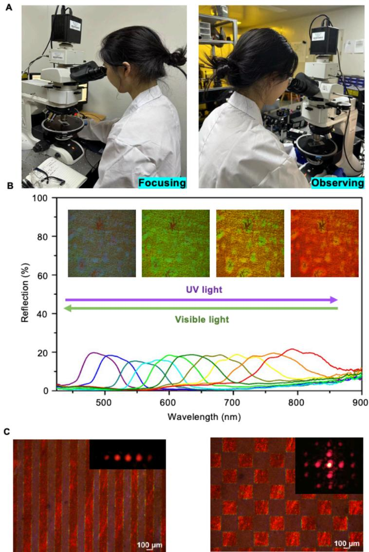
**Figure 2.4 Manipulating optical microstructures with broad-range structure color.** (A) Focusing the polarized optical microscope and observing the structures. (B) The spectrum of the photoprogrammable printing ink under UV light and visible light. (C) The microstructure textures of one-dimensional and two-dimensional gratings and the corresponding diffraction spots.
