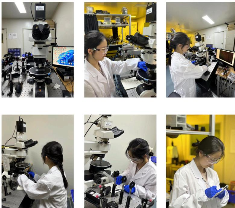
**Figure 4.2 Testing the optical performance: texture and spectrum.** From left to right, top to bottom: Polarized optical microscopy; Placing the sample; focusing; observing; recording the results.
