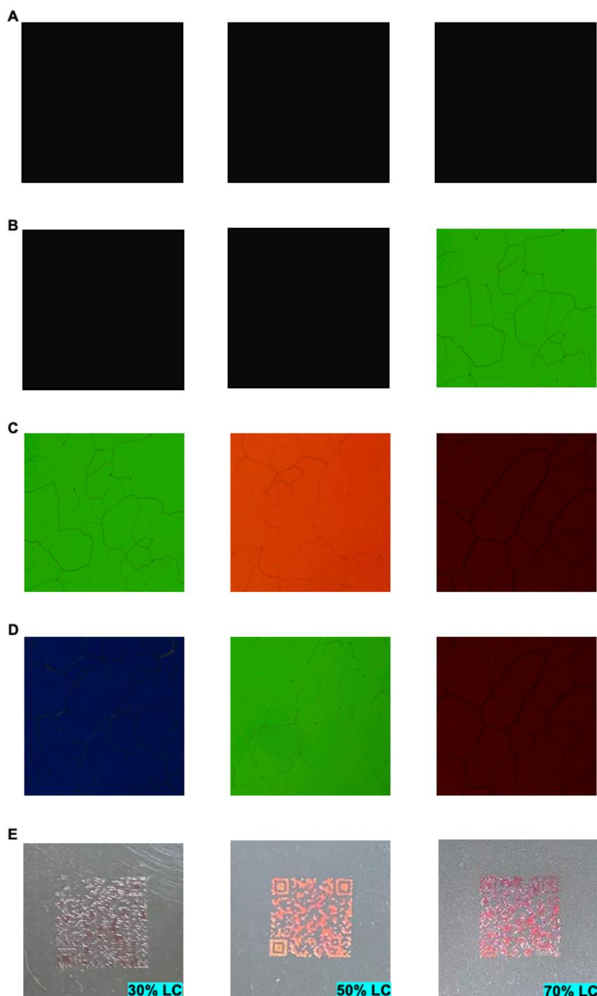
**Figure 2.2 Exploring the optimal mix proportion of photoswitch, liquid crystal and Polymer ink.** (A) 2.0 wt% of DAE in system showing reflection color range from green to red. (B) 4.2 wt% of DAE in system showing reflection color range from green to red. (C) 3.4 wt% of DAE in system showing reflection color range from green to red. (D) 3.8 wt% of DAE in system showing reflection color range from blue to red. (E) The three systems with different proportion of LC tested.
