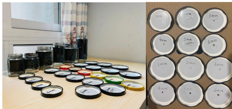
Figure 2.4: Part of the jars and caps with different hole diameter used in the experiments.
