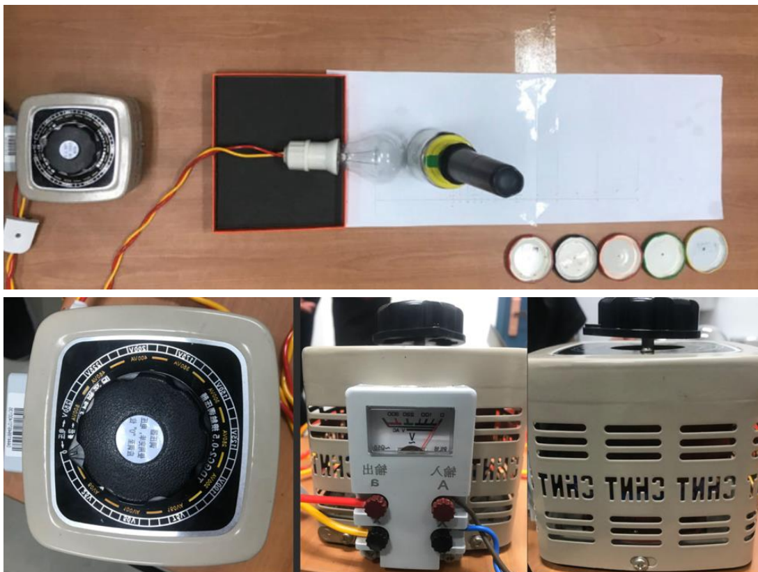
Figure 2.10 Experimental setup with the voltage transformer.
