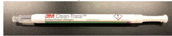
Figure 1.8 3M Clean-Trace ALLTEC60 for the detection of the presence of surface protein allergens
