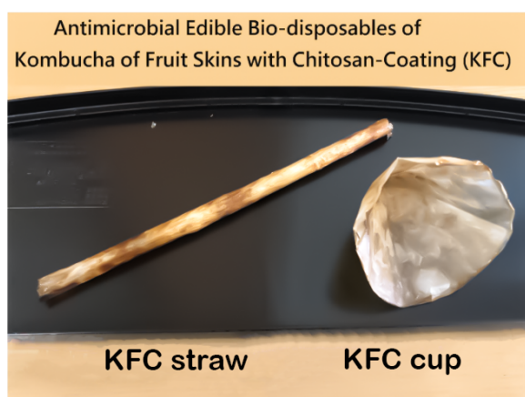
Figure 1 Antimicrobial edible bio-disposables of kombucha of fruit skin with chitosan coating (KFC) of orange skins of Fanel Supplement
