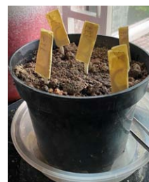
Figure 2.3 Investigation of the biodegradability of different samples in a pot of soil
