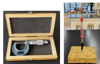
Figure 2.2.2. Measuring tensile strength using calliper micrometer (left) and spring balance (right)
