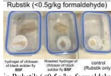
in Rubstik (<0.5g/kg formaldehyde) Figure 2.2.1.3 Measurement of concentration of HCHO removed by hydrogel of BSF
