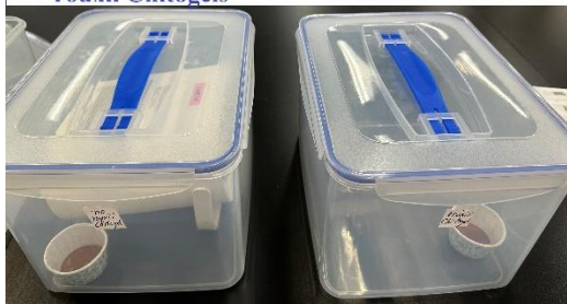
Figure 2.4.2 rouxii Chitogels as filter in an air purifier in a 9.3L air-tight box with 0.5g Rubstik 0.5g/kg HCHO)
