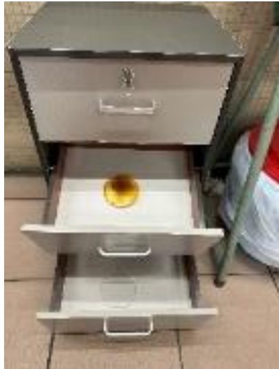
Figure 4.3.3 Anti-bacterial forma-ridden rouxii Chitogels as HCHO remover in new furniture of drawers emitting about 0.5 \text{ mg/m}^3 HCHO (exceeding safety limit of 0.125 \text{ mg/m}^3 )
