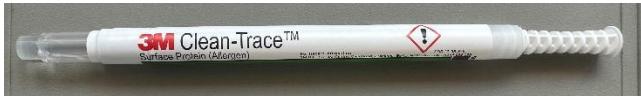
Figure 2.6 Detection of the presence of allergens in Chitogels and rouxii Chitogels of BSF using 3M Clean-Trace ALLTEC60 for detection of surface protein allergens
