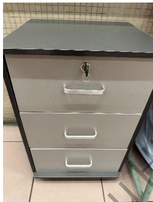
Figure 2.4.3 Furniture of drawers emitting about 0.5 mg/m 3 HCHO (exceeding safety limit of 0.125 mg/m 3 )
