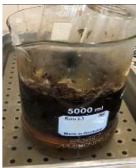
Figure 2.1.1.1.2 Deacetylation of chitin of BSF to chitosan
