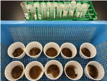
Figure 2.1.2 Dried hydrogel with different ratio of mass of hydrogel to volume of vinegar
