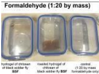
In 1:20 by mass of formaldehyde Figure 2.2.1.1 Measurement of concentration of HCHO removed by hydrogel of BSF
