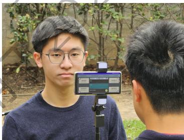
Figure 3: A visual demonstration of GazeLink converting eye gestures to sentences to facilitate communication
