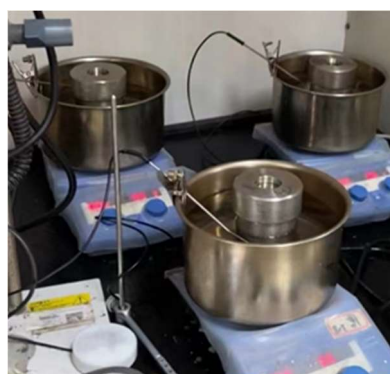
Fig. 2.2 Hydrothermal reaction system
