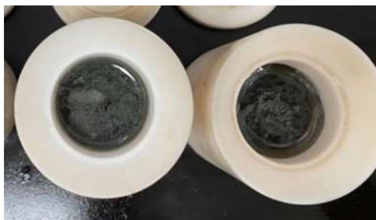
Fig. 3.6 \text{NTO}/\text{Ag}/\text{g-C}_3\text{N}_4 suspension by hydrothermal reaction
