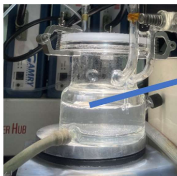
Fig. 3.13 Reactors with (a) Powder Catalyst and (b) Membrane Catalyst
