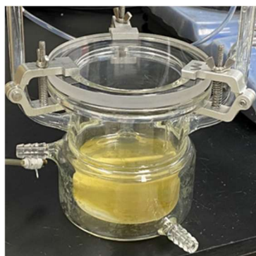
Fig. 3.13 Reactors with (a) Powder Catalyst and (b) Membrane Catalyst
