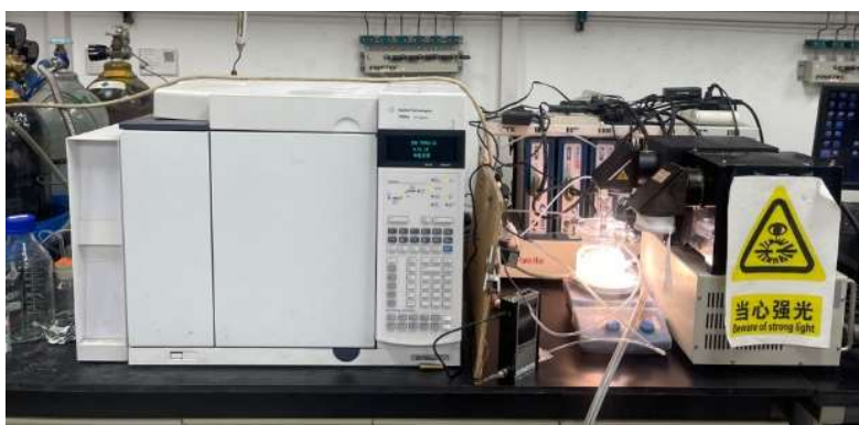
Fig. 2.5 Visible Light-Driven Hydrogen Production Setup
