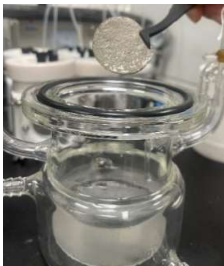
Fig. 3.15 NTO/Ag/g-C 3 N 4 membrane after a 3-h reaction
