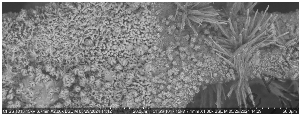
Figures 3.4 (g) and (h): \text{Cu}_x\text{Ni}_{1-x}\text{S} nanostructures (prepared by 1 mM \text{Ni}^{2+}(\text{aq}) and 120 °C hydrothermal heating) in atomic % (Ni/S) of 75% (left) and 50% (right) respectively
