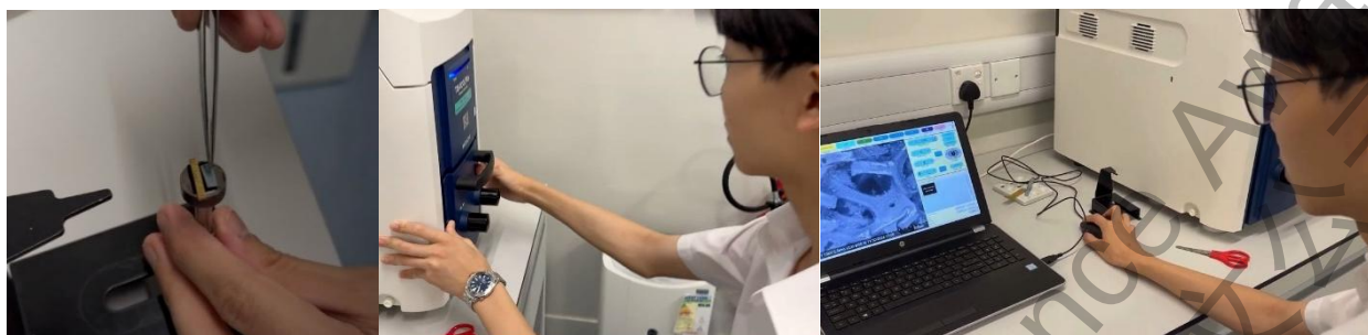
Figure 2.2 (a) Left: Mounting the sample for SEM analysis (b) Middle: Fixing the sample inside the vacuum chamber for degassing (c) Right: Samples under SEM analysis
