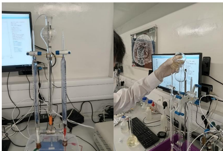
Figure 3.11 (a) Hofmann Voltammeter Set-up for hybrid water electrolysis of water (left). 1 M KOH or a mixture of 1 M KOH and 0.333 M urea are used as electrolyte (right).
