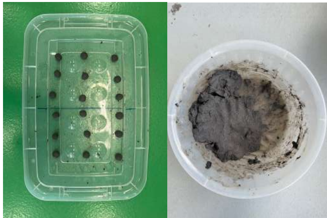
Figures 8.1 and 8.2. Soil mixing process, in which a small amount of water may be added to ensure homogeneity and form small spherical balls. The resulting 18 soil balls had an average mass of 5.01 grams (SD = 0.198).
