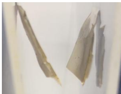
Fig. 72. Rupture of AC21 film after the bending strength test
