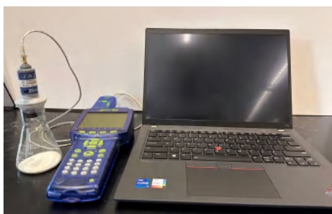
Fig.25. The set-up used to measure oxygen-absorbing ability of a sample
