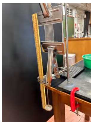
Fig.65. The experimental set-up used to assess tensile strength of the films.
